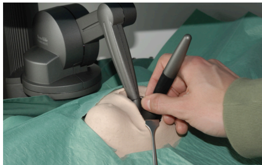
Fig. 3. Passive silicon and plaster mannequin and hand tool supports the activity in the simulator.
