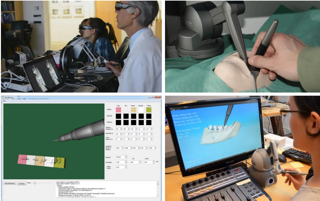
Figure 3. A) A surgeon teacher illustrating a surgical technique to medical students in an anatomy lecture. B) Mannequin used for hand support and for reference and context of dentistry. C) Screenshot from tool for setting and tuning the parameters modulating the feeling of carving, for a particular CG object. D) Midi-controller interface for tuning haptic sensation.
