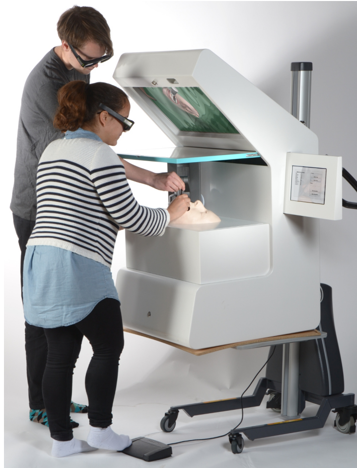
Figure 2.5: The Kobra Oral Surgery Simulator. Illustration of instructor and student solving a patient case.
