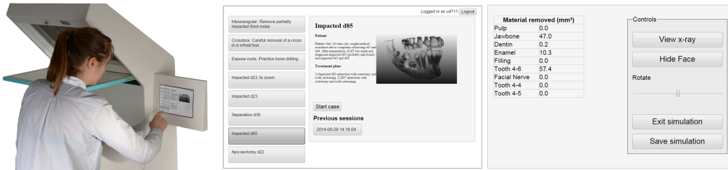
Fig. 4. The Graphical User Interface. a) interaction with the tablet computer b) case selection, c) display of how much volume is removed from each tissue layer and execution controls.
