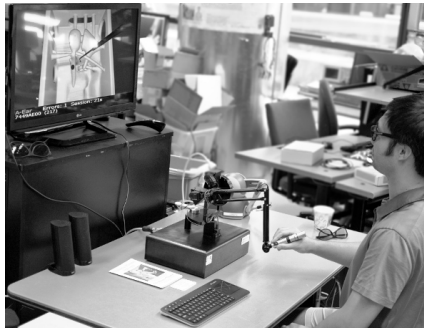
(a) Experimental setup showing the Phantom Premium 1.5/6-DOF haptic device and 3D television.
