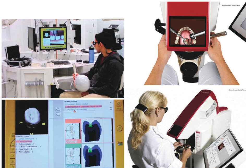
Figure 2.6: Left: DentSim simulator uses a passive mechanical simulator base coupled with optical tracking and on-screen visual feedback. Right: Simodont Dental Trainer. A wide-spread commercial dental simulator. DentSim video frame from image-navigation.com/mental-image accessed 2016-02-12, used with permission. Images of Simodont courtesy of Moog Industrial Group, used with permission.
