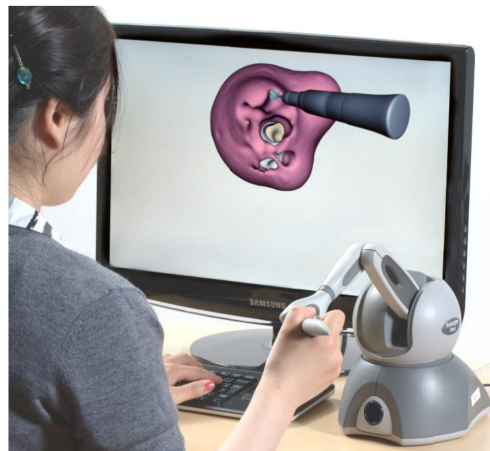
Figure 1. Carving in a solid, multi-layered computer graphics object with a virtual drill using force-reflecting haptic feedback in the process
